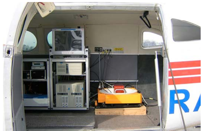
GSM 3000 mount with Zeiss LMK aerial camera system. The AEROcontrol IMU-IId is mounted on the adapter-ring.
