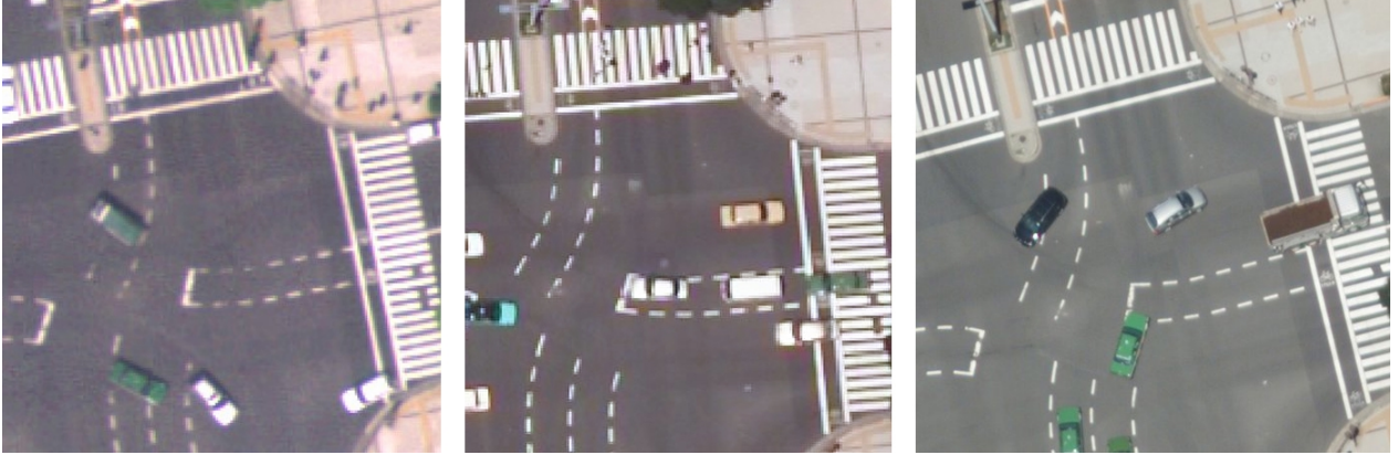
ADS40, GSD = 20 cm UltraCam D, GSD = 20 cm UltraCamD, GSD = 8 cm (Courtesy PASCO-Japan, owner of 3 “push-brooming” and 2 UltraCam-D)
